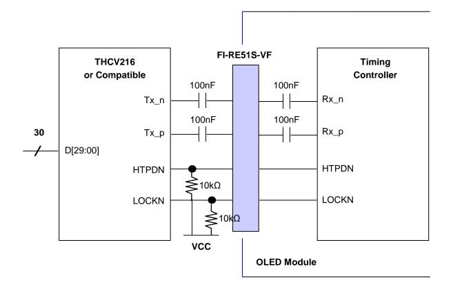
Note: 1. The OLED module uses a 100 nF capacitor on positive and negative lines of each receiver input.
