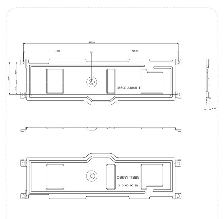
**NOTE** 1. Unspecified tolerance is  $\pm 1.0$ mm
